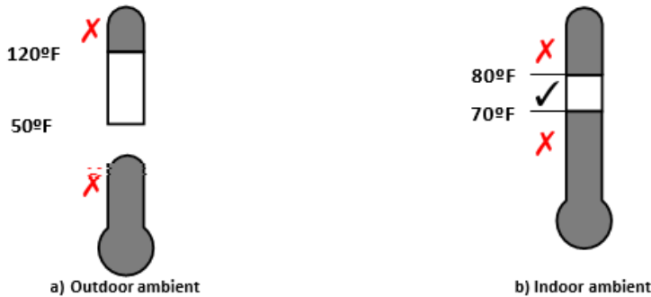
Figure 13-2 Temperature limit for AUTO charge mode
