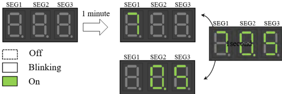
Figure 13-1 LED display in AUTO charge mode
